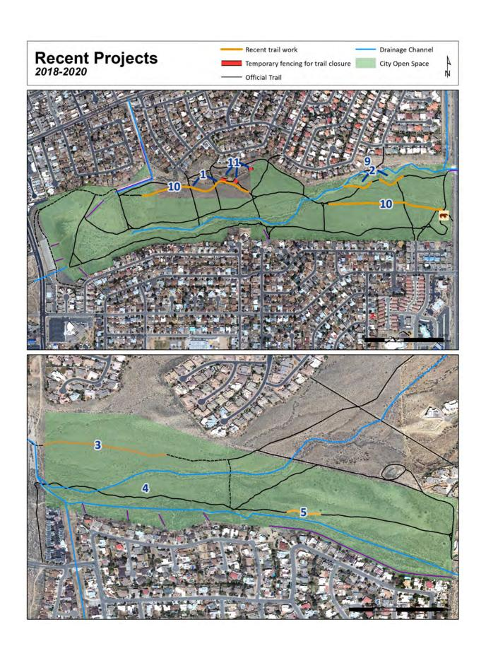
1. The OSD performed trail work on the private open space north of Bear Canyon West during October 2018 and July 2019, closing an eroding trail near incised drainage and formalizing a lower trail to form a connection across the private open space. There are two access points on the private open space at
